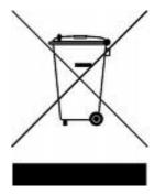
The wheelie bin symbol now displayed on equipment supplied by Geotechnical Instruments signifies that the apparatus must not be disposed of through the normal municipal waste stream but through a registered recycling scheme.
